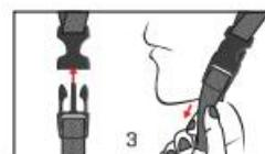
A SISAK VISELESE KÖZBEN NYOMJA ÁT A SISAK EGYIK FELET A MÁSRÉLÉ. HÜZZA MEG A HEVEDEREKET, HOGY MEGBIZONYOSODJON ARRÓL, HOGY A CSATOK MEGFELELŐEN VANNAK RÖGZÍTVE, ÉS HOGY A RÖGZÍTÖRENDSZER RÖGZÍTVE VAN. LÁSO NO.3
